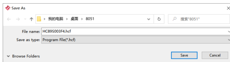
Figure 4.8-2 save file dialog box, select the save path and click the "save (s)" button to save the burned file to the local disk
